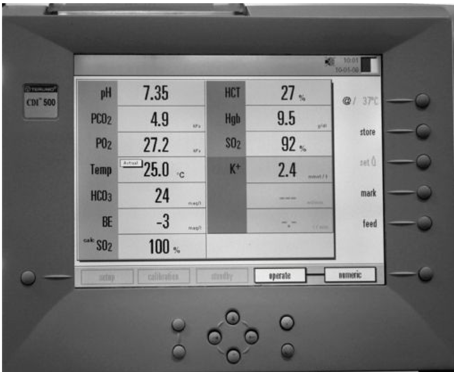
Figure 1.14 Terumo CDI 500 in-line monitoring system, providing real-time blood gas, acid/base, Hb/HCT, and electrolyte analysis.
