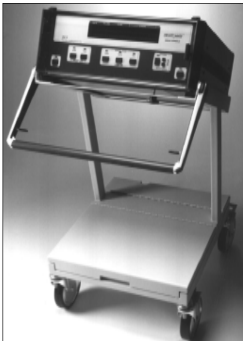
Fig. 2.12. The Thermo Cardiosystems 1000 IP LVAS pneumatic drive console. (Photograph courtesy of Thermo Cardiosystems, Inc.).
